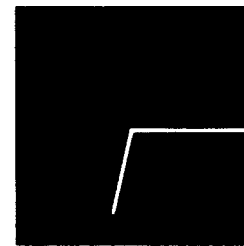
Diode in series with 51 \Omega
